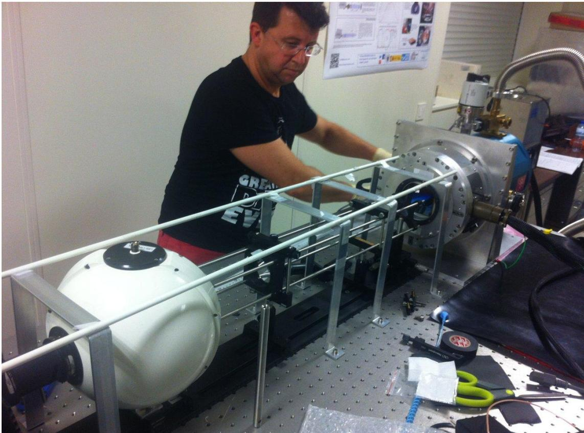
*Figure 21: PSF measurement setup.*
