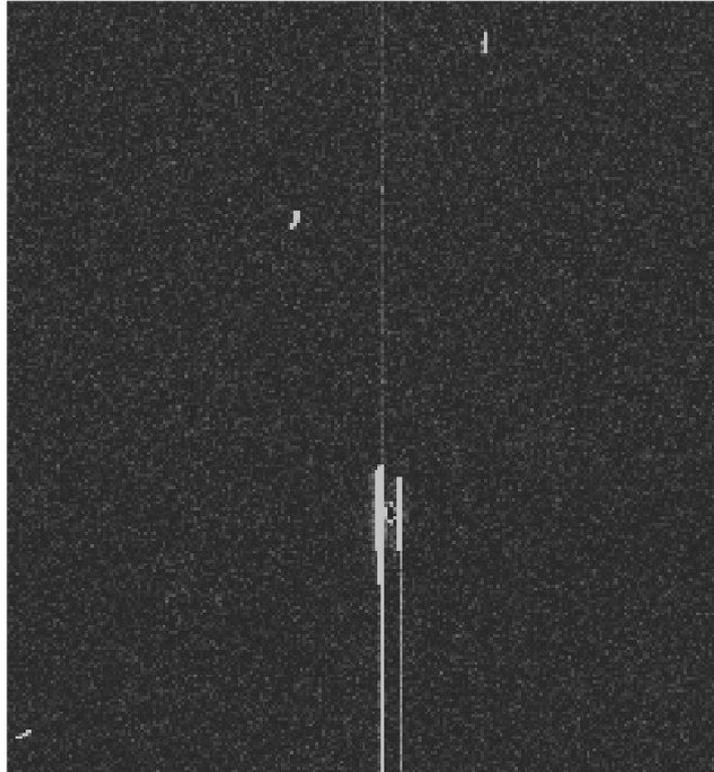
**Figure 14:** Cluster of defects visible in quadrant E (centred on  $x=2561,y=3118$ )
